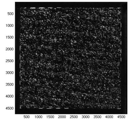
The array shown here has features in a  $640 \times 640$  grid, for a total of 409,600 features. Each feature represents a 25-bp probe.
