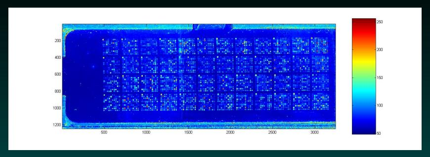
As we have seen previously, glass microarrays are typically laid out in a hierarchical layout, containing a rectangle of grids, each of which is a rectangle of spots. Also, each grid is spotted on the array by a different physical pin.
