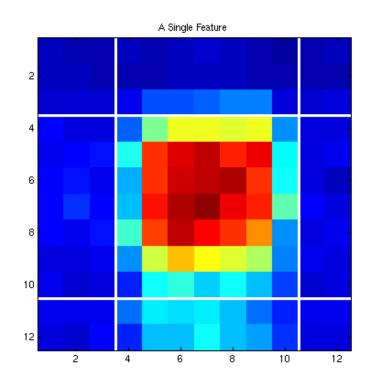
Each feature on this chip is approximately 7 pixels (20 microns) on a side. In general, Affymetrix features use many fewer pixels than are used for the round spots in the images of other types of microarrays. Features are not perfectly uniform!
