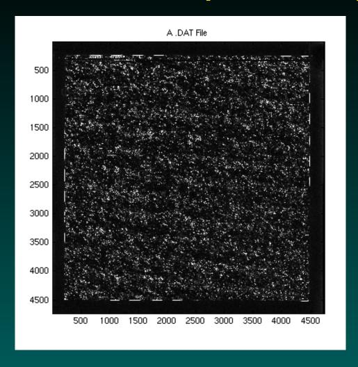
The array shown here has features in a  $640 \times 640$  grid, for a total of 409,600 features. Each feature represents a 25-bp probe.
