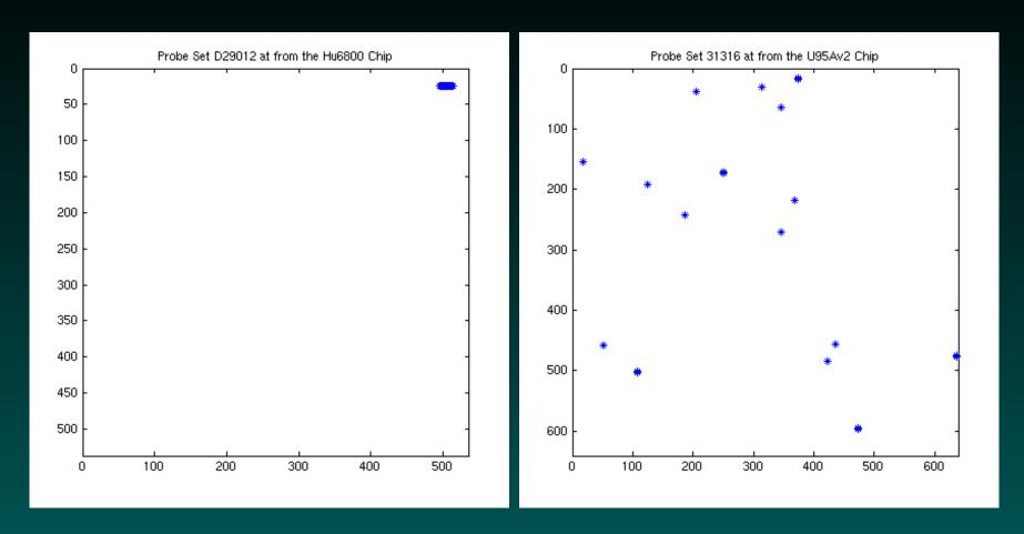
Probe set locations change with the chip type. In older chips, the probe pairs were adjacent. In newer chips, they are randomized.
