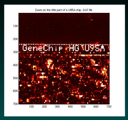
The pixelated features have been combined with positive controls to spell out the chip type – this helps ensure that the image is correctly oriented. Also note the border lattice of alternating dark and bright QC probes, making image alignment and feature detection easier.
