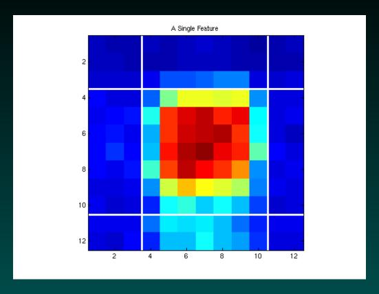
Each feature on this chip is approximately 7 pixels (20 microns) on a side. In general, Affymetrix features use many fewer pixels than are used for the round spots in the images of other types of microarrays. Features are not perfectly uniform!
