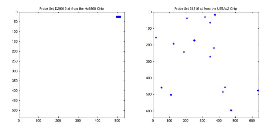
Probe set locations change with the chip type. In older chips, the probe pairs were adjacent. In newer chips, they are randomized.
