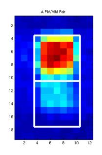
Affymetrix tries to control for cross-hybridization by coupling multiple probes that should work paired with those that shouldn't. These are known as the Perfect Match (PM) and Mismatch (MM) probes, and constitute "probe pairs".
