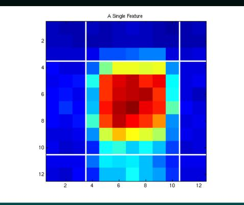
Each feature on this chip is approximately 7 pixels (20 microns) on a side. In general, Affymetrix features use many fewer pixels than are used for the round spots in the images of other types of microarrays. Features are not perfectly uniform!
