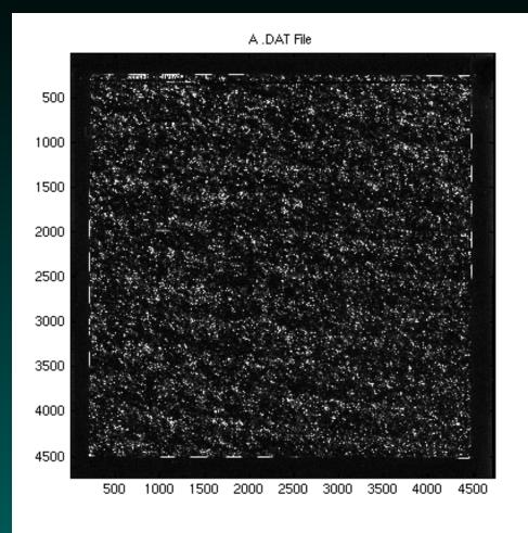
This array has a  $640 \times 640$  grid of "features" (409, 600 total). A "feature" has many copies of one 25-bp seq.
