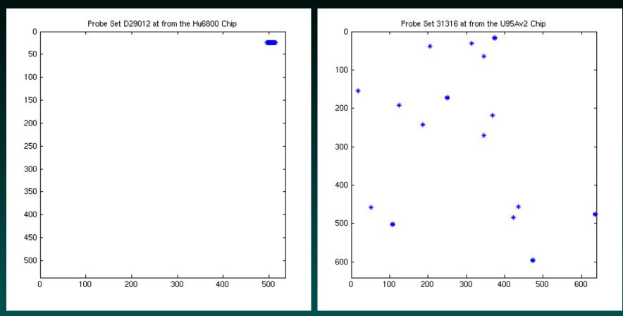
Probe set locations change with the chip type. In older chips, the probe pairs were adjacent. In newer chips, they are randomized.
