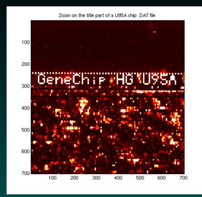
The pixelated features have been combined with positive controls to spell out the chip type – this helps ensure that the image is correctly oriented. Also note the border lattice of alternating dark and bright QC probes, making image alignment and feature detection easier.
