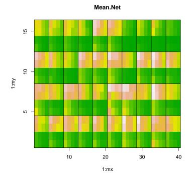
By default, image will use "Mean.Net" as the measure. Different spots on the array are separated by white lines, and different subgrids (patches) are separated by black lines. Here, we can see that the top 2 rows in each patch are different than the bottom 2 rows. To see how big the difference is, let's add a colorbar:
